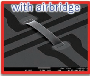
Image 2. Photograph of wire crossing with airbridge in the pseudo 2D network
