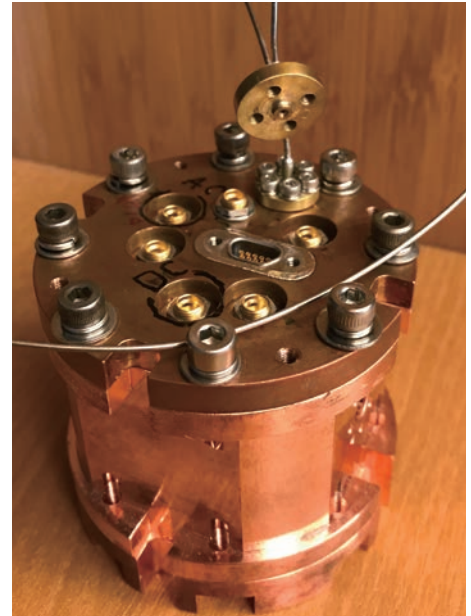
Experimental apparatus called "cell" to store liquid helium
